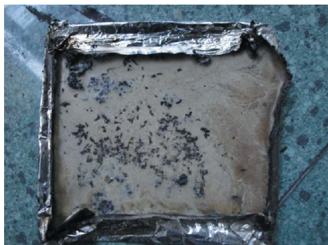
Figure 11 Photograph of residue under char of PP/20%IFR. [Color figure can be viewed in the online issue, which is available at wileyonlinelibrary.com .]
